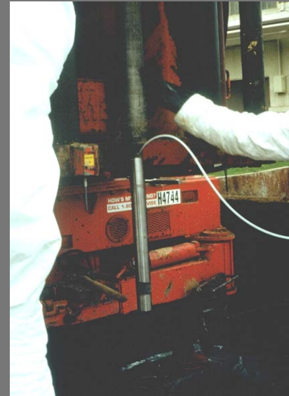
Mini Probe Soil Gas – Chlorinated Hydrocarbons, BTEX, Castle AFB – Used With Hollow Stem Auger
