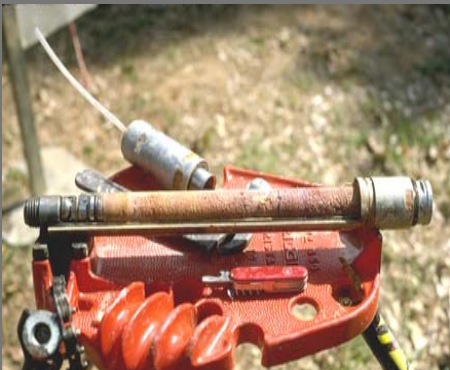
Mini Probe Soil Gas – Pima County AZ Landfill – Chlorinated Hydrocarbons – Used With Air Rotary Casing Hammer
